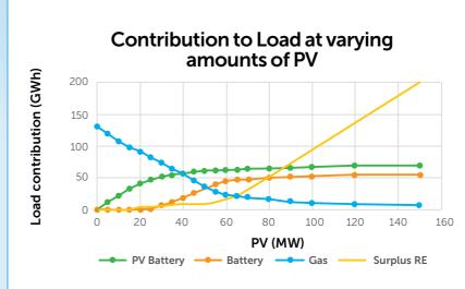
An electricity system has to meet the load put on it by consumers. This figure shows the contributions to meeting load across the year for PV, Battery and LNG, as well as the surplus (or spilled) generation as the amount of PV increases. Gas use decreases steeply to approximately 60MW of PV. PV's direct contribution to load increases steeply to around 20MW, after which increasing amounts are passed into the battery storage.
