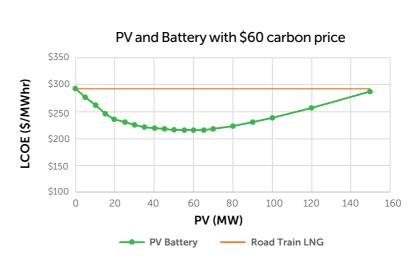
This figure shows the trend in LCOE for a range of PV capacities, with a carbon price of \$60 per
